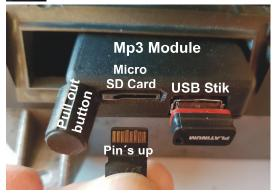
Insert the (short) USB stick, or the micro SD card into the module. For the micro SD card, the contacts must face up. Insert the micro SD card into the slot, push it in carefully until it clicks into place. To remove, tap on the SD card, this springs out of the slot.
